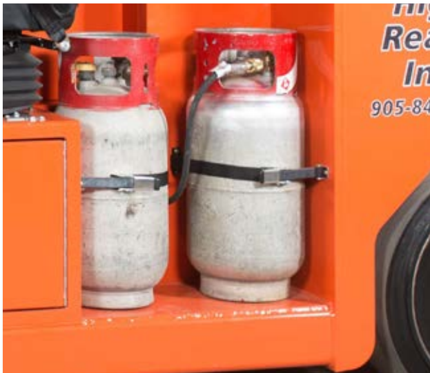
Very Low Lift LP Tank Loading. Improves safety immensely
