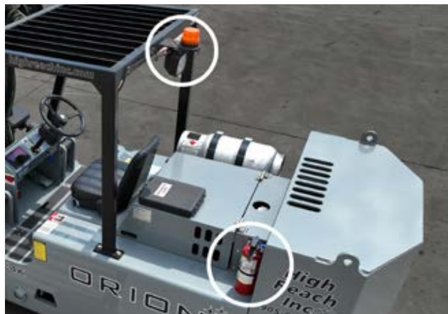
Back up alarm, in-operation strobe, among the safety features standard.
