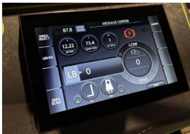
State-of-the-art electronic easy-read load scale.
