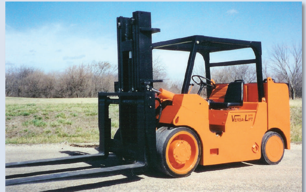
Versa-Lift 25-35: 35,000 lbs capacity
